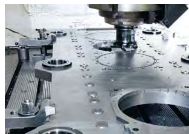
For stripper plates, the notches for the various elements of the tool are milled out.
