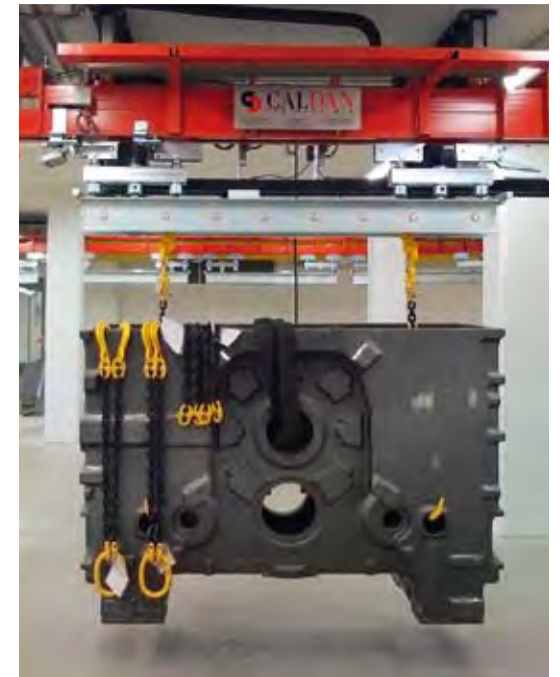
Parts weighing up to 2.5 tonnes are fed via massive rails through the wet painting system.
