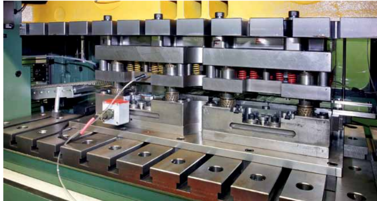
The two die sets mounted in-line (right for blanking and left for forming) allow to produce earthing strips from coil in one continuous operation.
