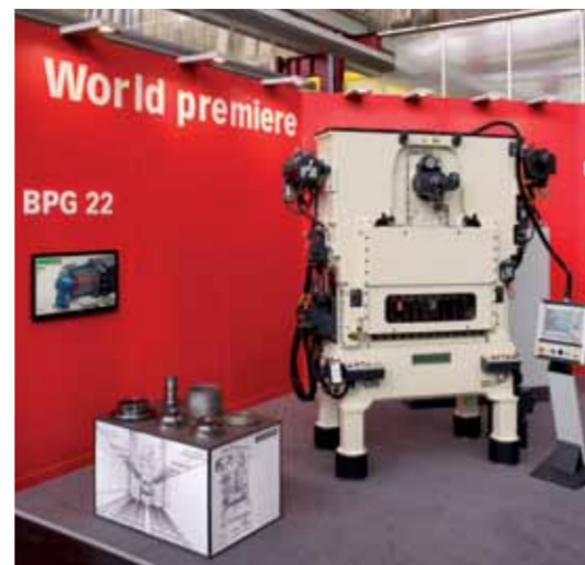
The newly-developed BRUDERER BPG 22 planetary gearbox fitted onto a BSTA 510-125.
