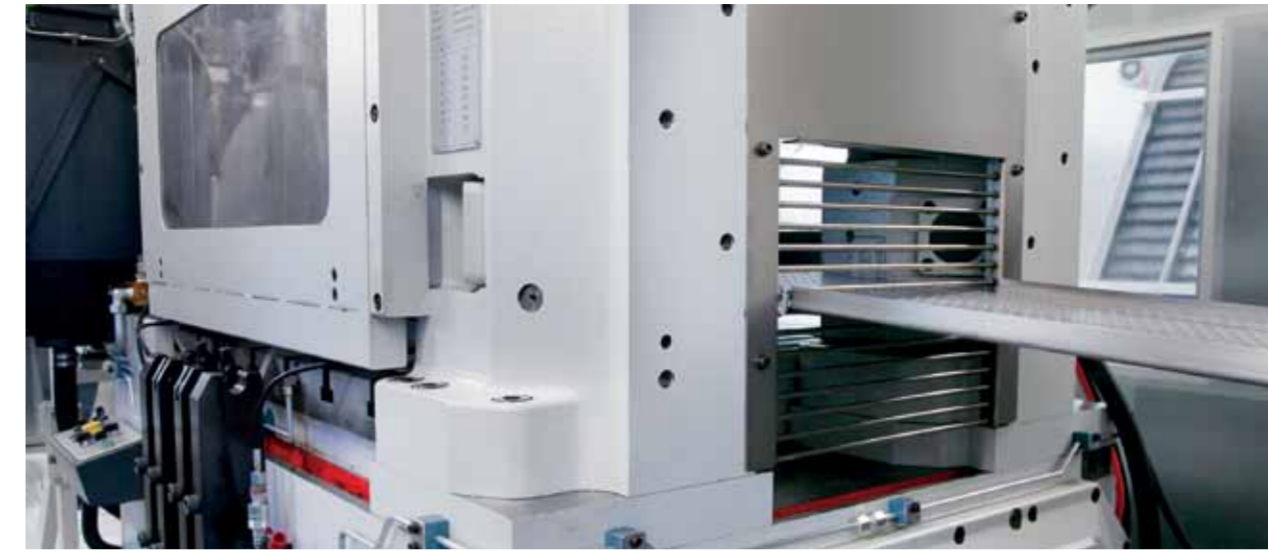
The strip remaining after the punching process is fed onto the reel using an ARKU re-winder.
