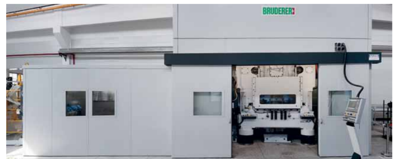
The BSTA 1600-117 produces coin blanks with the utmost precision and efficiency behind the doors of the sound-proof cabin.
