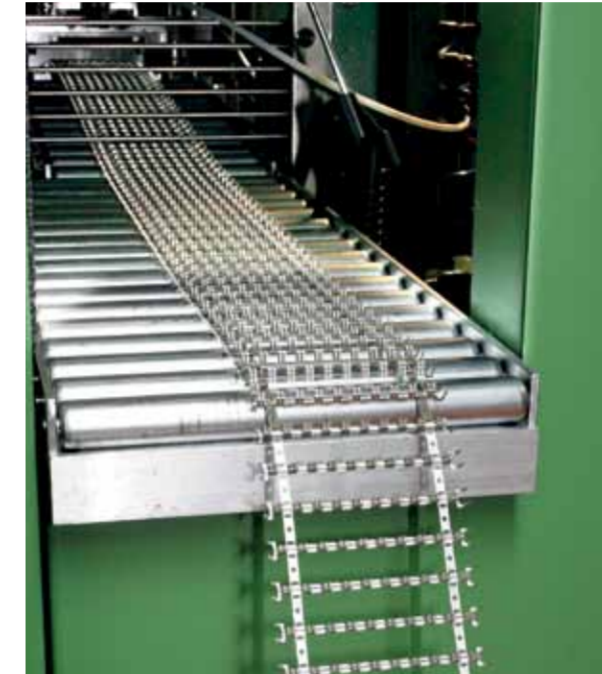
Up until now, the tin-plated copper earthing strips had been produced on smaller machines.
