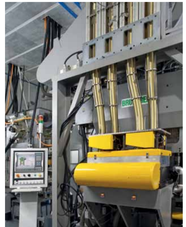
The stacked shells are fed into the BSTA 1250-117 for the conversion with the tabs.
