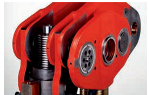
Ram adjustment during operation under production conditions.
