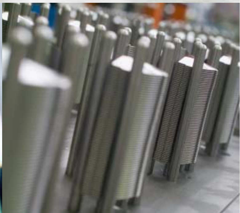
Production line for the blade manufacturing at DaimlerChrysler which has been delivered by BRUDERER. It contains a BSTA 80B from BRUDERER, decoiler and straightener from ARKU, tooling from WALTER POTTIEZ and the automatic cutting & stacking system from SEF // BRUDERER process control type B // Automatic cutting and stacking system // Automatically stacked blades //
