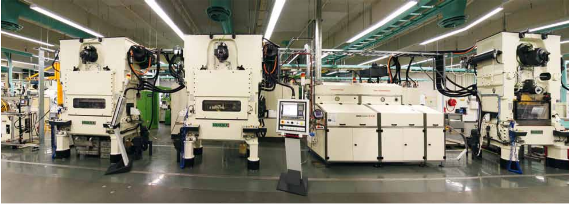
Networked automated punching presses provide maximum manufacturing efficiency for moderate costs.
