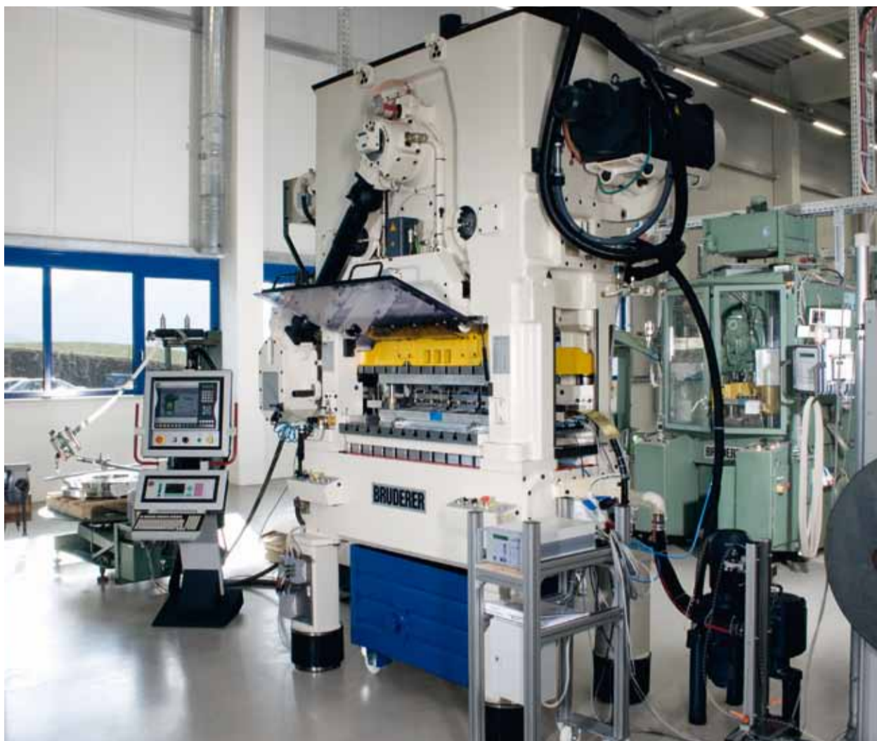
Various work-steps integrated into one process: Bruderer automated punching presses at Unimet.
