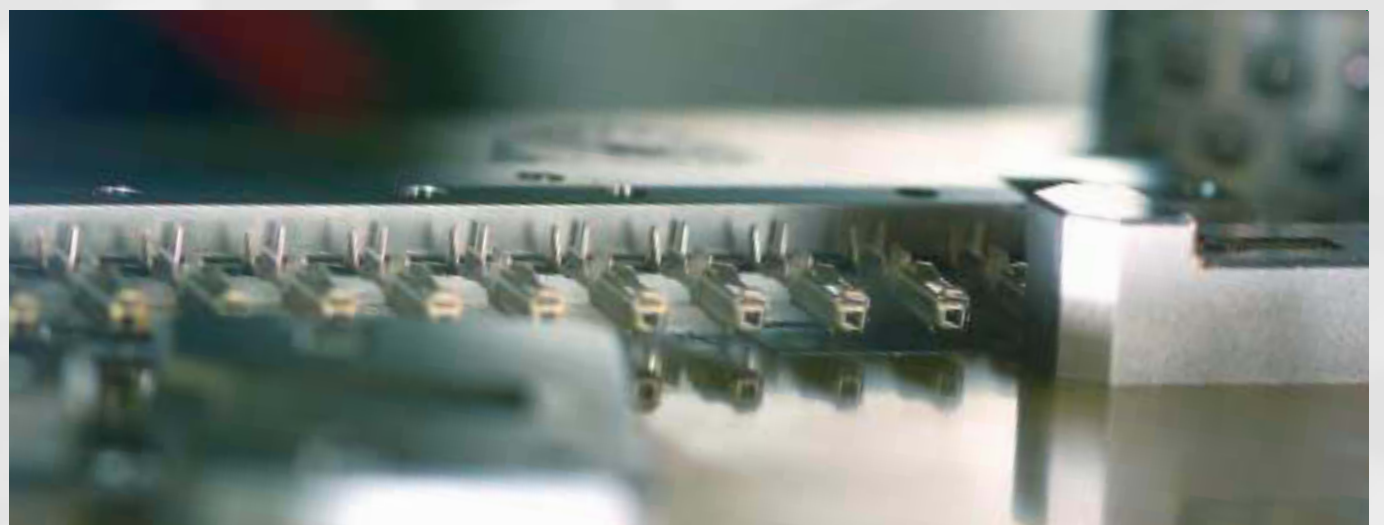
The result of a complex Two-Track production: highly precise contacts at the outlet of a STEPPER-die //
